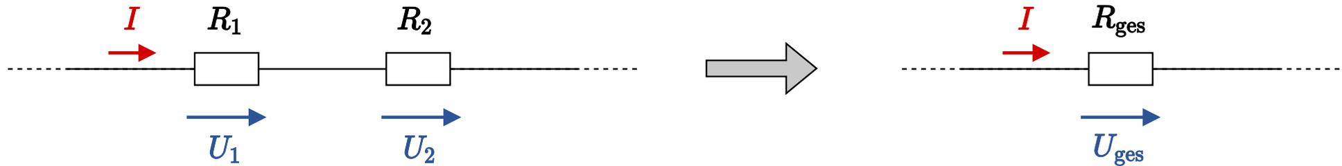
$$U_{\text{ges}} = U_1 + U_2 \quad \text{mit} \quad U_1 = R_1 \cdot I \quad \text{und} \quad U_2 = R_2 \cdot I$$
